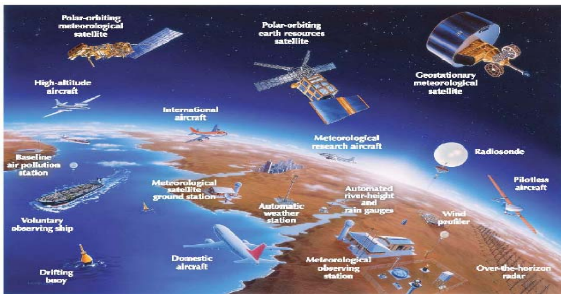
Figure 4.1 Schematic showing a variety of observation systems of relevance to National Meteorological and Hydrological Services. Observation networks rely heavily on the cooperation of many individuals and organizations, many of them volunteers. (Source: Bureau of Meteorology, Australia)
